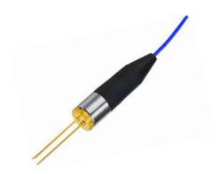
The FPLD series fiber-coupled laser diodes are designed with a GaAs quantum well structure. These diodes feature a built-in photodiode for precise monitoring and feedback control of the laser's output power. Housed in standard TO packages, these diodes are pigtailed to a 1-meter long single-mode fiber terminated with an FC/APC connector. Each unit undergoes rigorous testing prior to shipment to ensure reliability.
